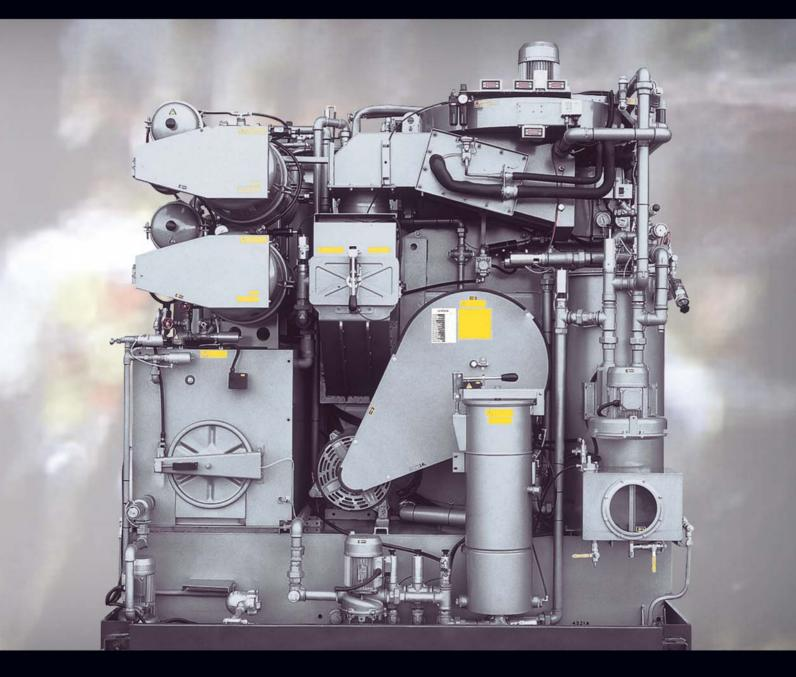
Logical, ergonomically designed for convenient, easy access to all components for quick maintenance. Multiple, independent spin disc EcoFilters™ and carbon cartridge filters.
