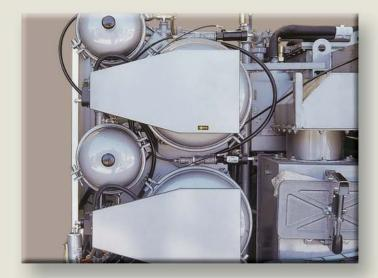
Multiple, independently functioning high-micron self-cleaning spin disc EcoFilters and large-capacity carbon cartridge filters are standard on all Union 800 Series Systems to assure optimum filtration of both large and small particles for maximum solvent purity. Computer controls automatically pair filter operation for whites, darks or colors according to specific programs.
